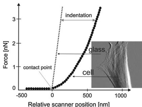
**Fig. 1** The idea of the Young’s modulus determination based on the subtraction of curves recorded on stiff (in our case glass coverslip) and compliant (dermal fibroblasts) surfaces
